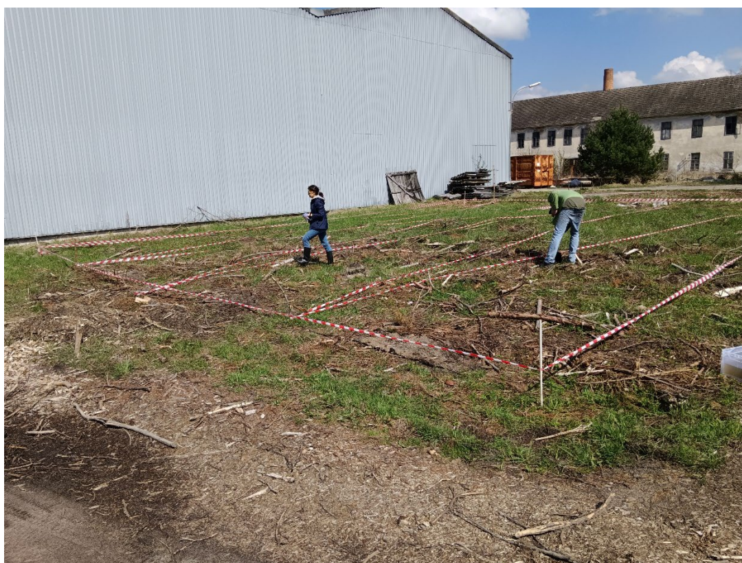
Figure 24: Marking out the test plots and the soil-sampling pattern for a representative composite sample for laboratory analysis.
